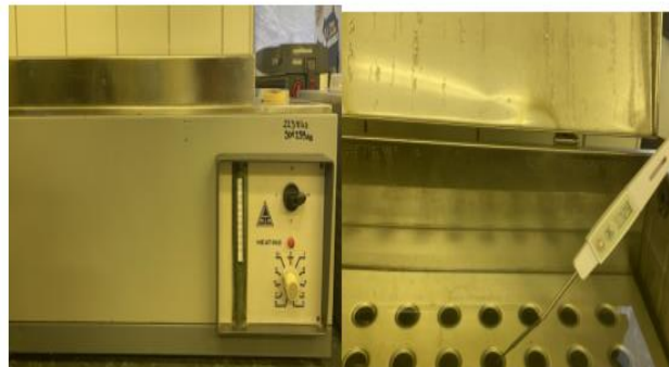
Figure 5. Thermostated water bath of 72°C detected by a hand-held thermometer
