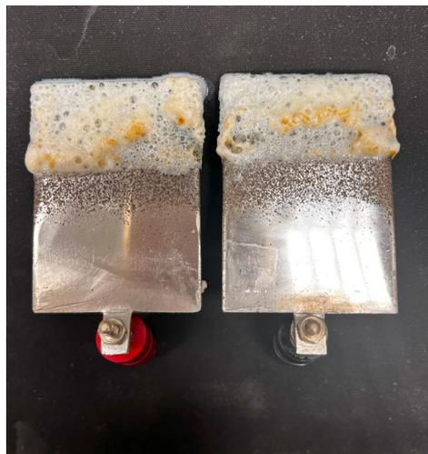
**28. Figure** The electrodes with the fat and whey aggregates after the hydrolysis
