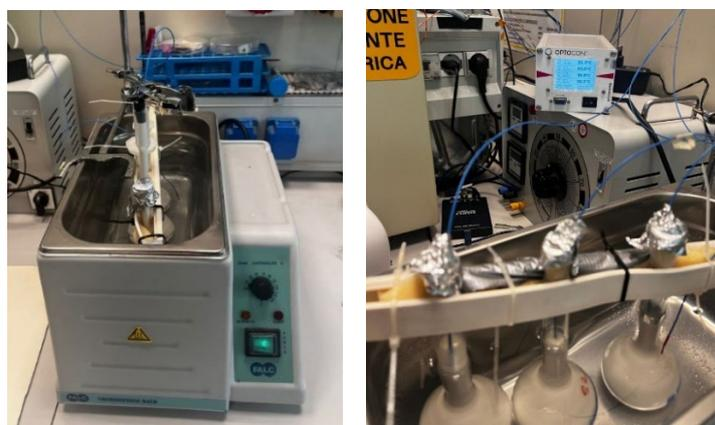
**22. Figure** Enzymatic hydrolysis in water bath and system for the temperature monitoring and control of individual samples and of water bath
