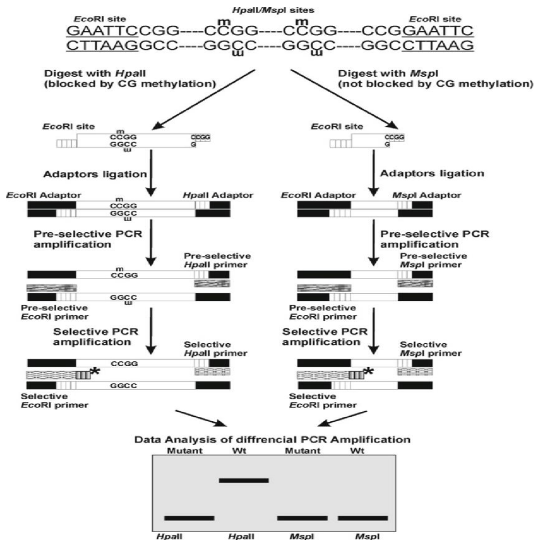
Figure 7: Illustration of the MSAP procedure: Initially, DNA is subjected to digestion with methylation-sensitive ( HpaII ) and methylation-insensitive ( MspI ) endonucleases, followed by the ligation of the resulting DNA fragments to particular adaptors. Subsequently, these ligated DNA fragments are employed as templates in an initial PCR reaction utilizing specific primers. The resulting PCR products are then utilized as DNA templates in a subsequent selective PCR reaction, employing three selective nucleotides as fluorescently labeled primers (indicated by asterisks).
