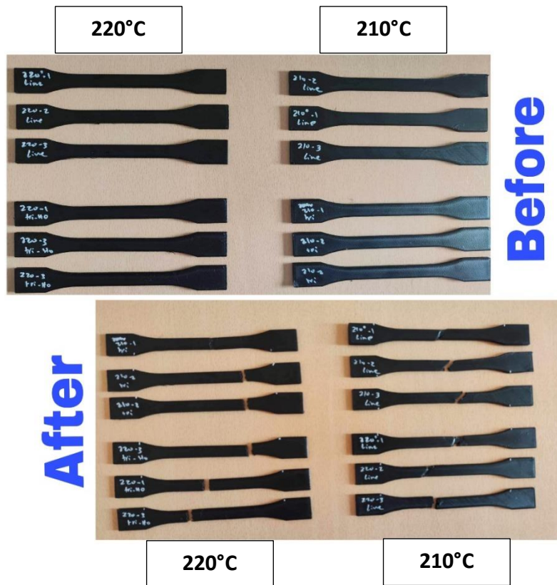
Figure 20: Line and Tri-hexagonal samples with different printing Temperature
