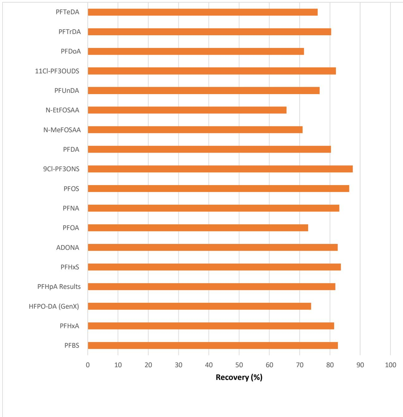
Figure 14. Optimized recovery results of SPE.
