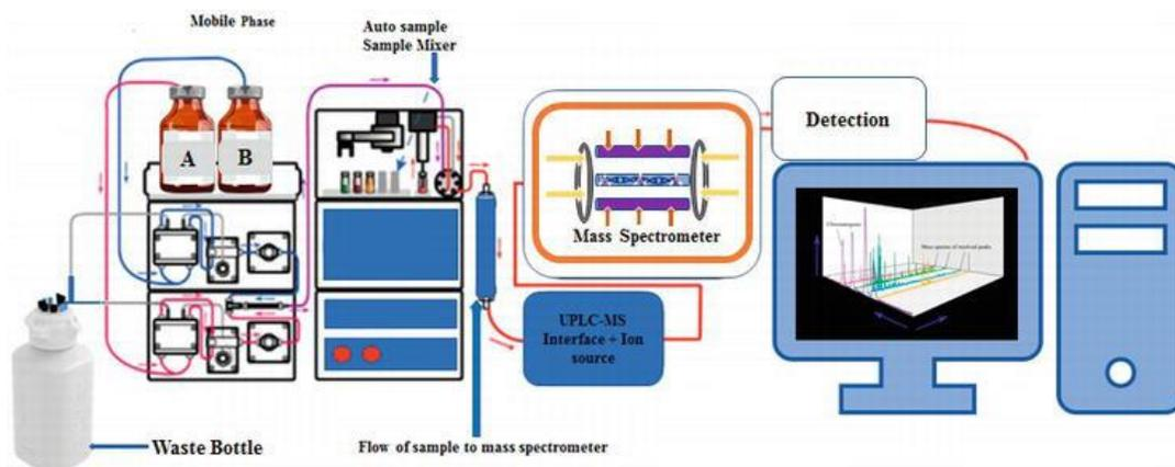
Figure 7. Flow diagram of ultra performance liquid chromatography-mass spectrometry (**Ashraf et al., 2020**).
