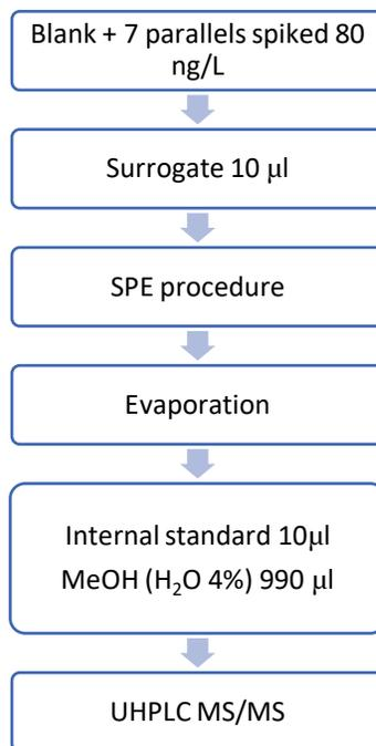
Figure 8. Experiment steps for the demonstration of SPE sample preparation accuracy and precision.
