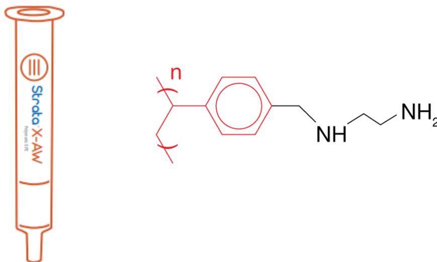
Figure 5. Strata-X-AW SPE and the chemical structure of its cartridge surface (**Phenomenex, 2023**).
