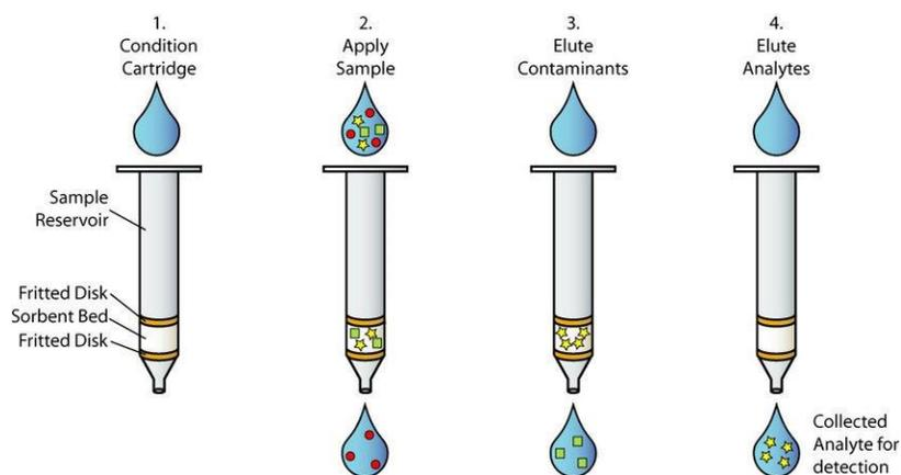
.Figure 6. The Solid Phase Extraction Syringe (**Hawach, 2024**).
