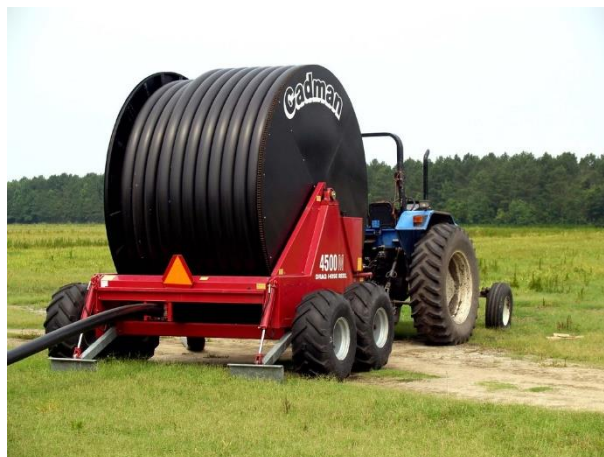
Figure 5: Hard hose reel irrigation system
