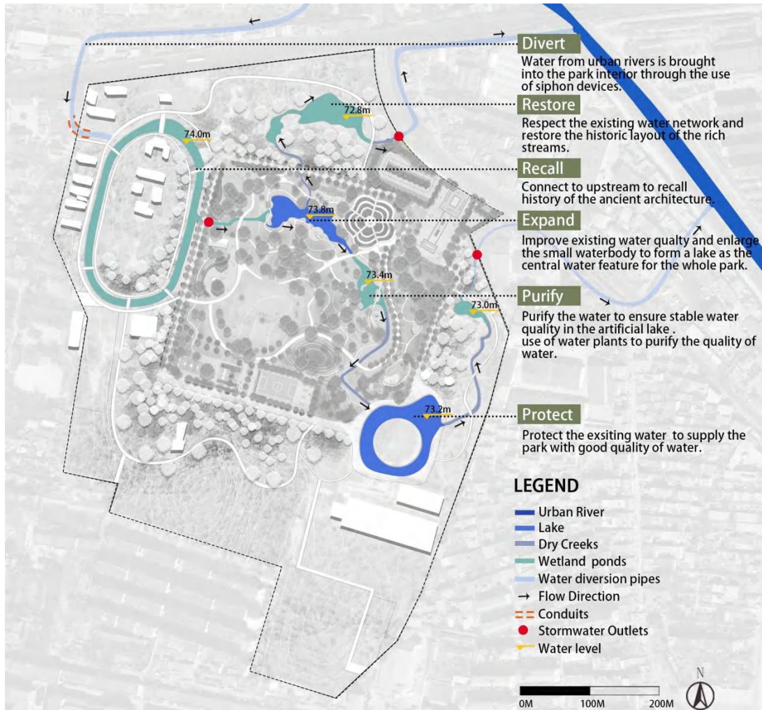
(Figure 5-18) Water System Ecological Design Diagram
