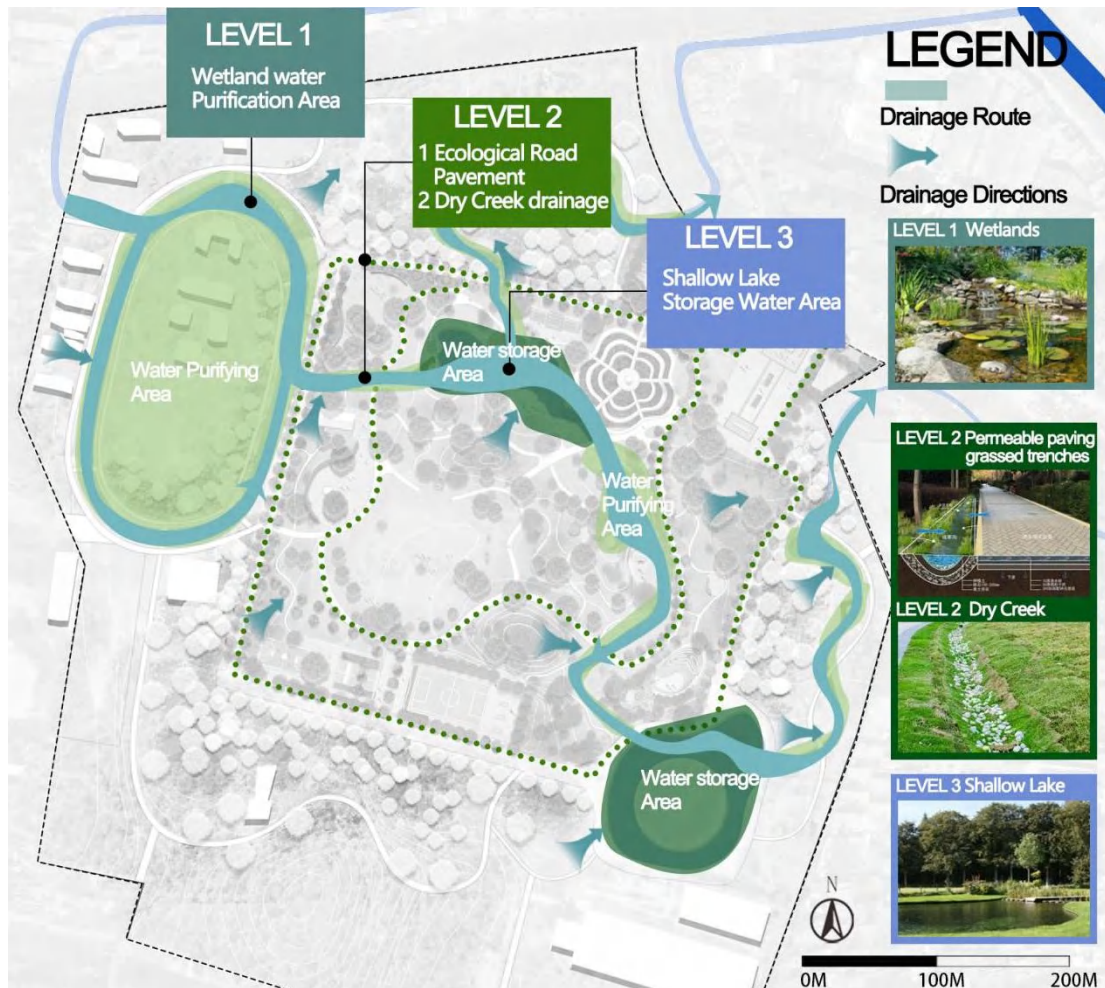
(Figure 5-19) Drainage Ecological Design Diagram
