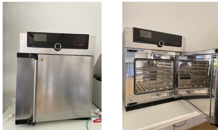
Figure 15: The machine was used to get dry slum gum in 60°C (Photo: Kim 2023)
