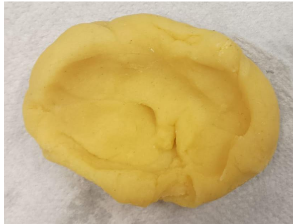
Figure 16. Picture of Corn flour Type 2 after kneading with adequate amount of water.
