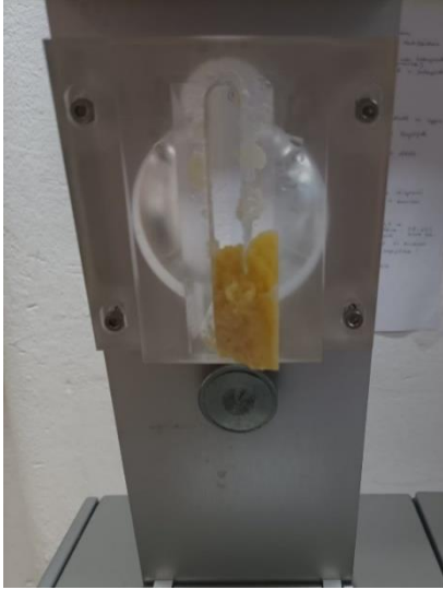
Figure 18. Piece of corn dough stuck on the lid at the beginning of kneading.
