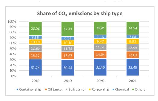
Figure 8 - Share of CO<sub>2</sub> emissions by ship type
