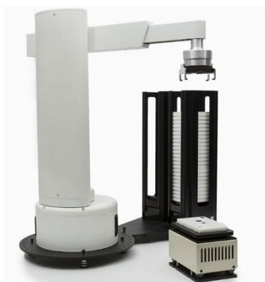
Figure 3. A cylindrical robot arm [5]
