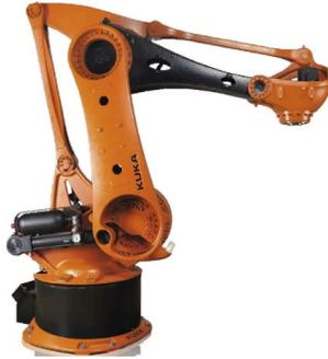
Figure 6. Kuka Articulated robot KR 700 PA [21]
