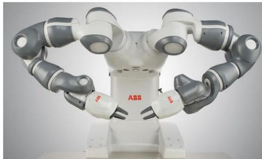
Figure 2. YuMi, a collaborative robot developed by ABB. [4]
