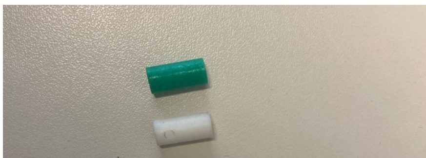
figure 3.1 PTFE and PE HD 1000 cylindrical specimens that were used in the pin-on-disc tests (source: MATE, Tribology lab)
