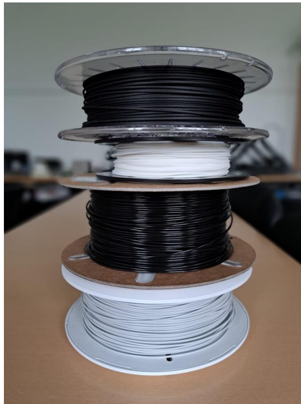
Fig 18. PLA Filaments : HD PLA Fiberlogy, rPLA 3D JAKE, PLA White CREALITY, and PLA Carbon Spectrum. (bottom to top)
