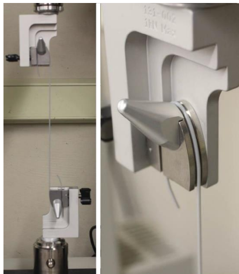
Fig 11. PLA filament testing using Bollard style grips(left), lose up of clamping method (right).[45]
