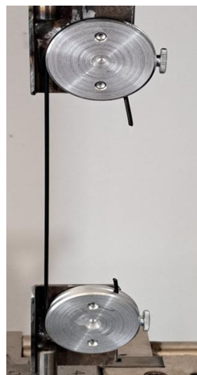
Fig 41. The filament testing using the bollard style tensile grips.
