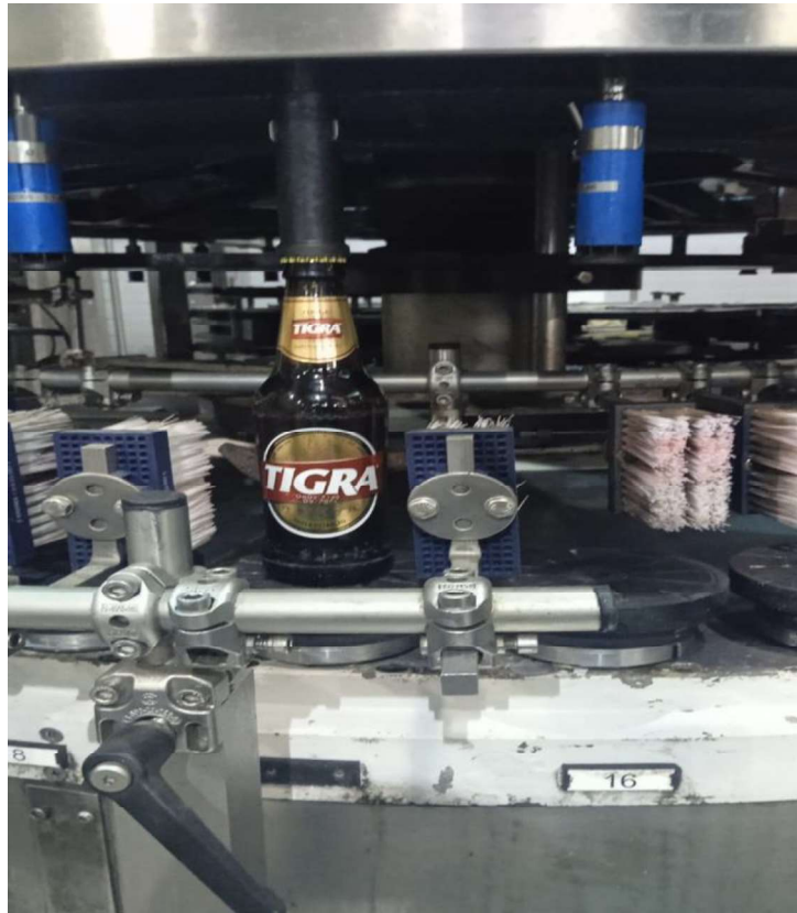
Figure 23 - Labeling machine repaired with replacement of new servomotors.
