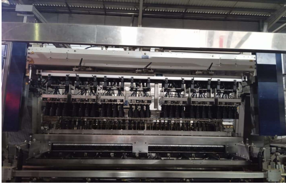
Figure 21 - Degrader and crater head straightened and slides centralized in the box center.
