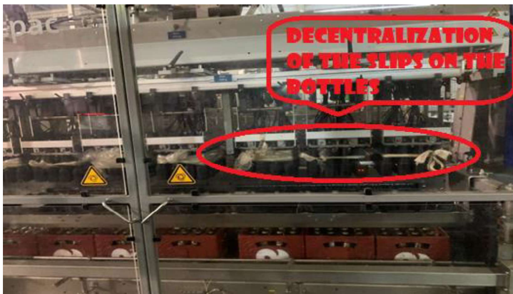
Figure 15 - Grader and degrader with the lids decentralized on the bottles, the operators tie cloths to centralize.
