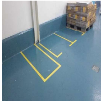
Figure 64 - After visual marking of pallets and pallet trucks on the line.
