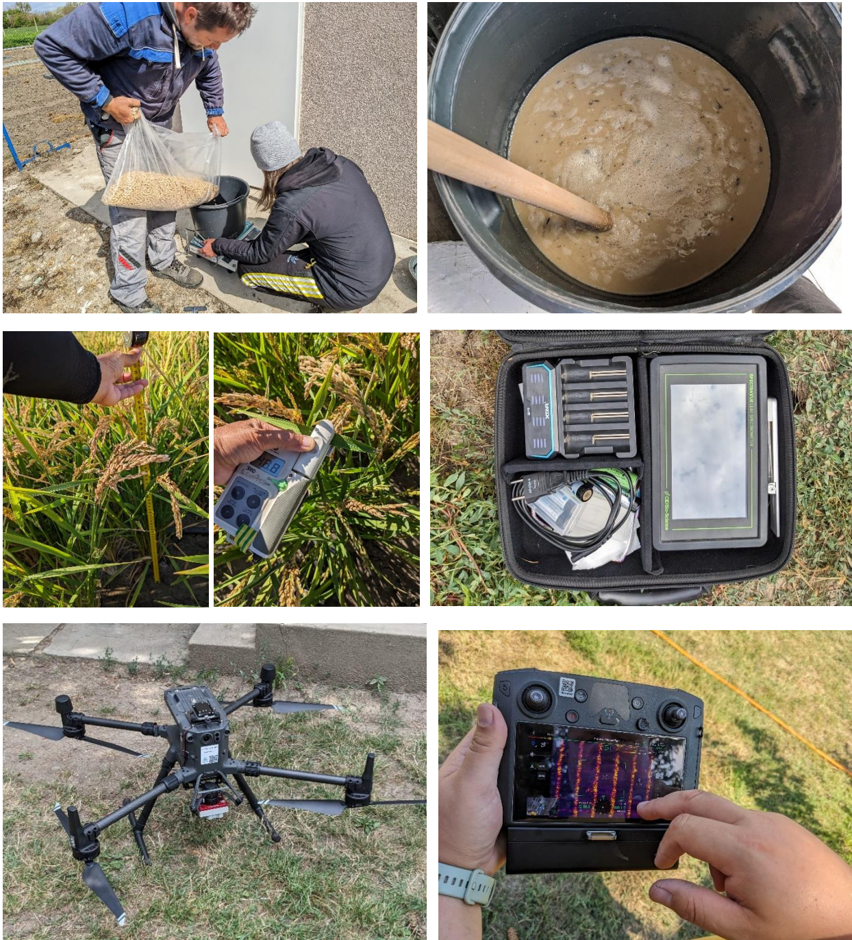
Appendix 1: Preparation of organic fertilizer (top); Rice plant measurement using a measuring tape (mid-left), SPAD chlorophyll meter (mid-middle), and SpectraVue leaf spectrometer (mid-right); UAV devices used in taking the multispectral and thermal images of rice (bottom).
