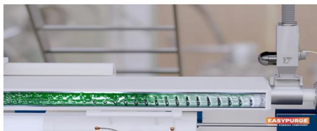
Figure 2.2.4 How liquid purging compounds chemical agents react inside the barrel. (Andres Rodriguez 2020b)
