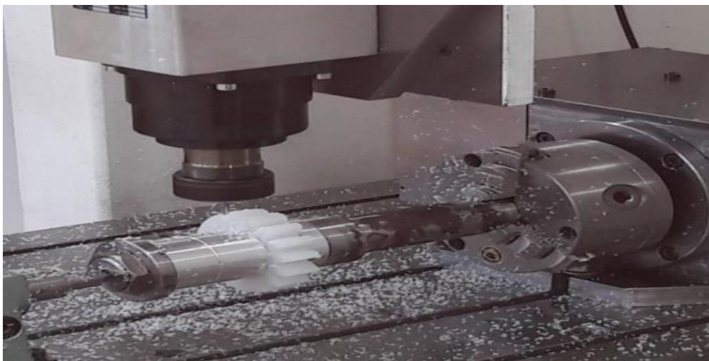
Figure 6: Milling process for polymers (Lie, 2019)
