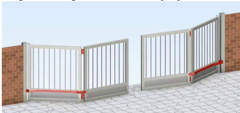
Figure 16 Bi-folding gate moving from the closed position [27]
