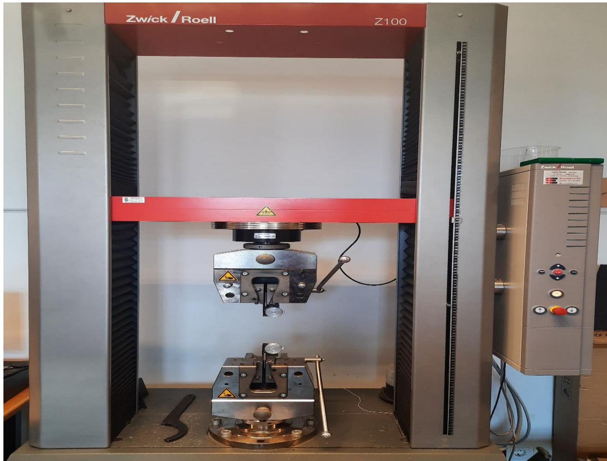
Figure 25. Zwick Z100 materials testing machine
