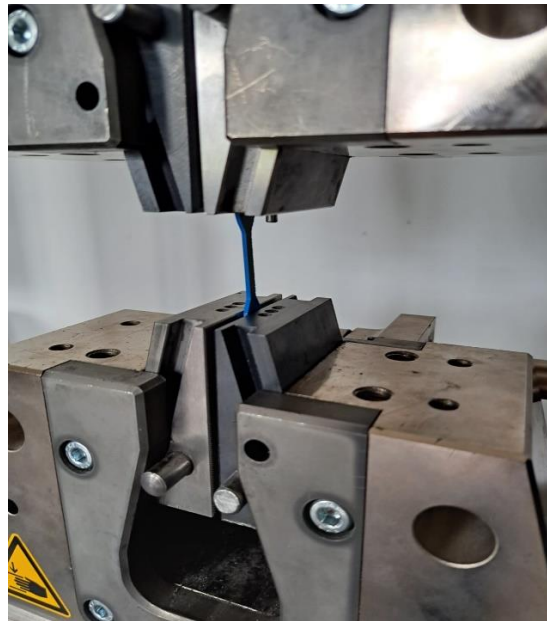
Figure 28. Tensile test of the printed PETG standards
