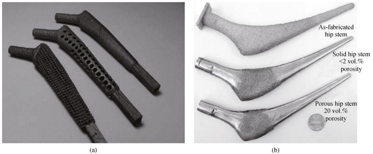
Figure 16. (a) Hip stems with mesh, hole and solid configurations fabricated using EBM (Source: [40]); (b) functional hip stems with designed porosity (no porosity, <2 vol.% porosity, and 20 vol.% porosity) fabricated using LENS (Source: [41])
