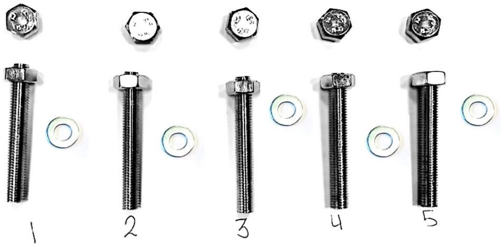
Figure 47 Group B of M10 bolts have a 5.8 yield strength with washers and locking nuts
