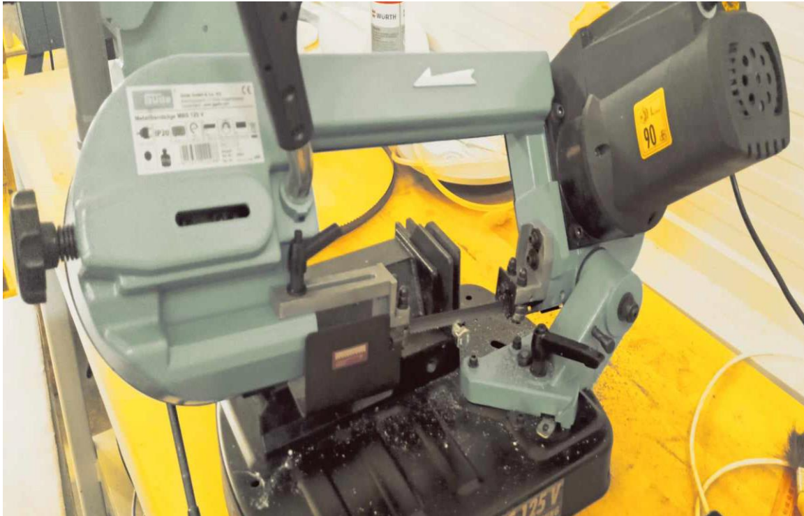
Figure 39 Electric cutting machine for cutting bolts-head before the experiments
