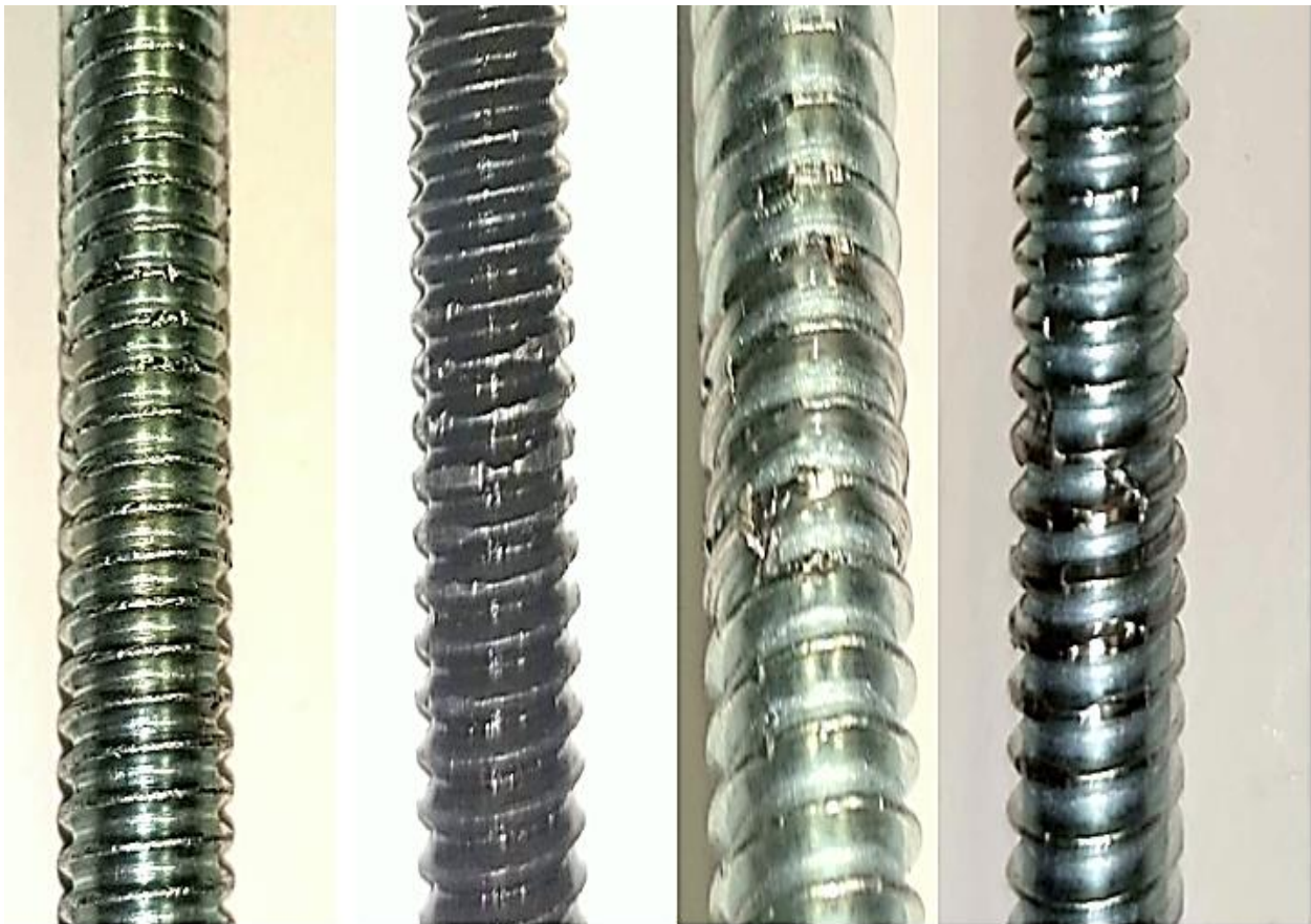
Figure 53 Frictional effects on the thread contact area of M10 bolt
