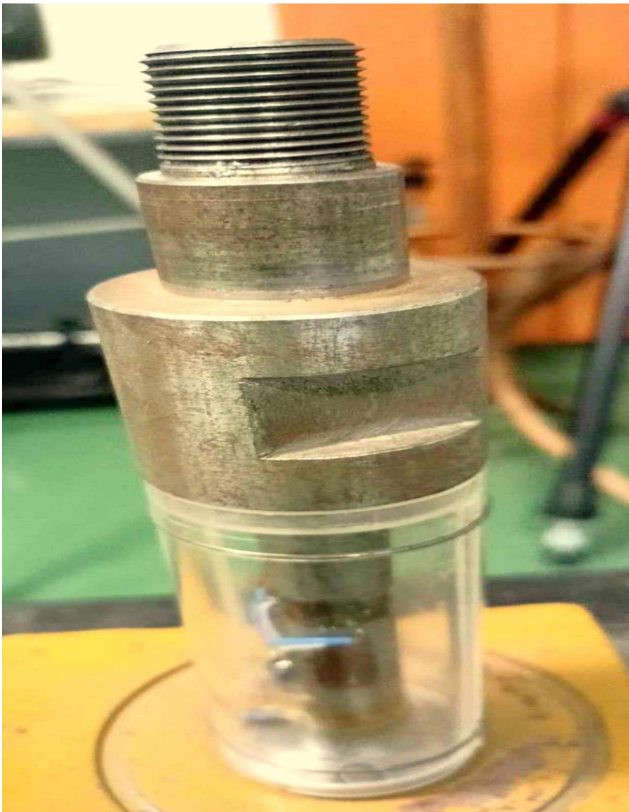
Figure 27 Measuring screw with the strain gauge sensor inside part of the measurement device
