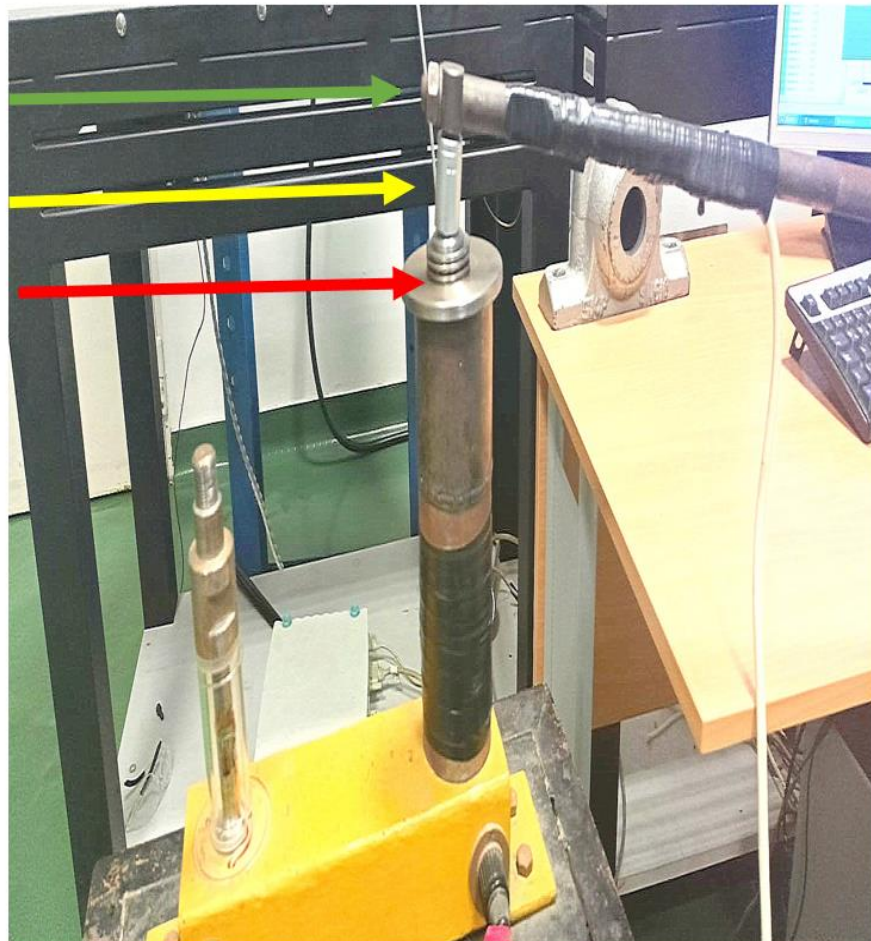
Figure 44 testing the coefficient of friction of M10 Bolts device setting up with applied bearing
