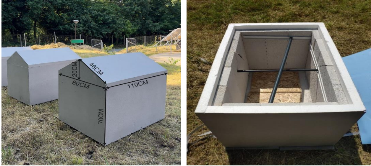
Figure 8. a) Dimensions of model house. b) Interior components of model houses.
