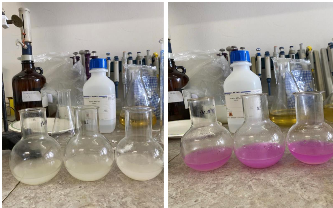
Figure 18. Free-fatty acids titration of ultrasound assisted extract powder mixed with sunflower oil
