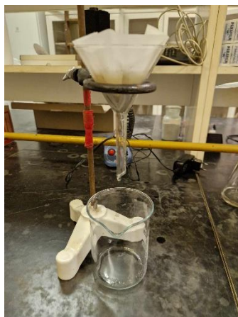
Figure 13. Separating soil/sediment phase from the water phase through a glass funnel with a paper filter and a holder
