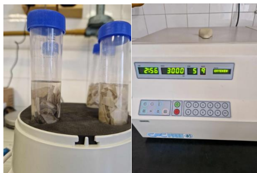
Figure 14. Paper phase analysis in 50mL centrifuge tube and centrifugation instrument
