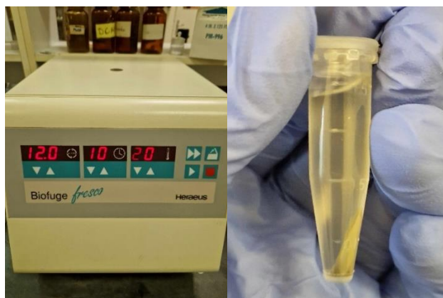
Figure 12. Eppendorf centrifuge instrument and Eppendorf tube containing separated solid phase and water phase
