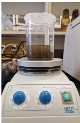
Figure 11. Stirring the solution with magnetic stirrer and stir bar
