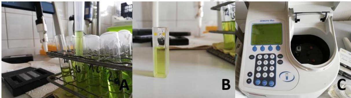
Figure 15. Leaf pigment measure by spectrophotometry. A: cube charge by pipette. B: cube charged for measure. C: measure of 644, 663 and 480 nm wavelengths by GeneSys VIS-10 spectrophotometer
