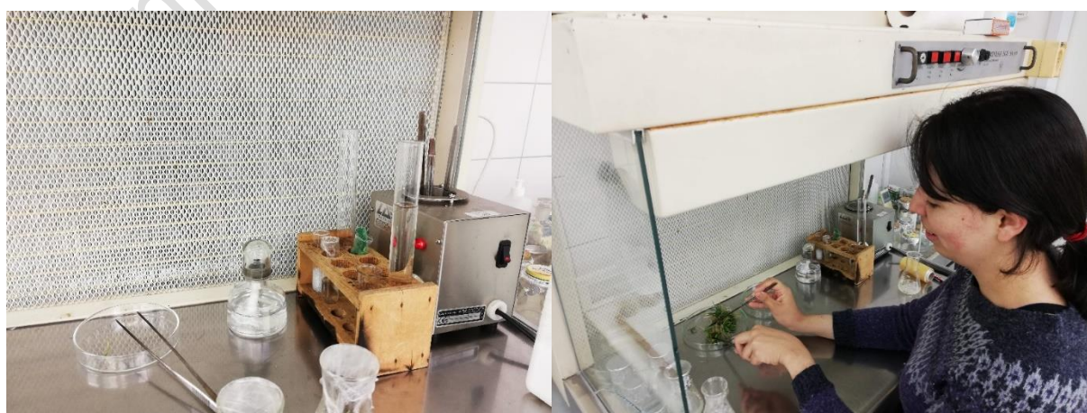
Figure 2. Sterilized materials, tools (left), and laminar flow cabinet as workspace (right) to avoid contamination
