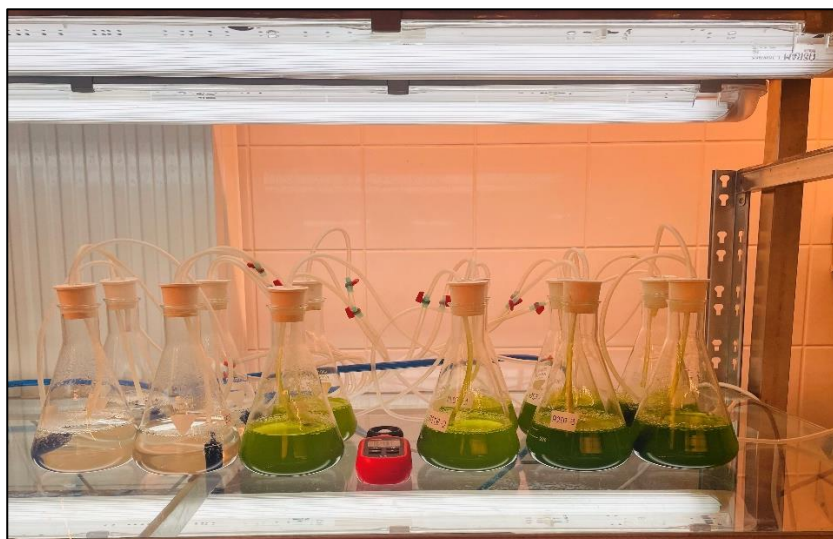
Figure 5: Algae growth in 500mL flasks supplied with air and illuminated with fluorescent lightning
