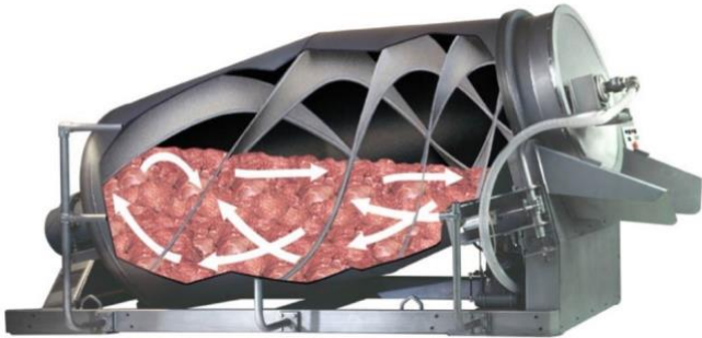
Figure 7. Meat tumbler (cross section) (Internet source 2)
