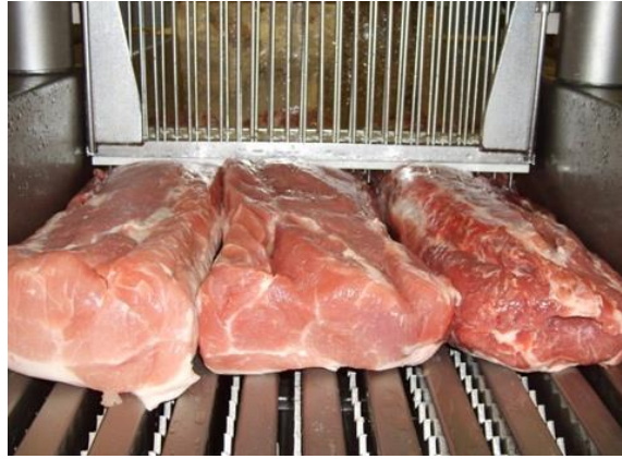
Figure 6. Injection curing of the pork loin (Meats and Sausages ©, 2022b)
