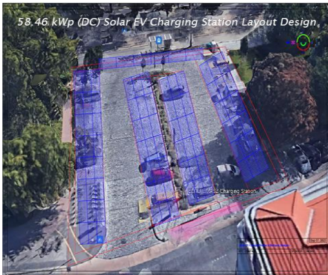
Figure 2: Ground-Mounted Model Solar EV Charging Station Layout, [Own Work, Software: AutoCAD]
