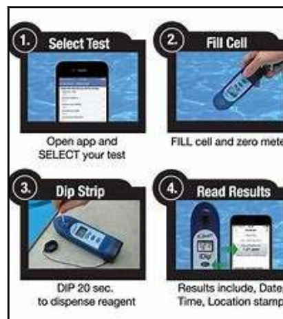
Figure 11. eXact iDip Smart digital Photometer Testing Steps Source: Web 3, n.d.
