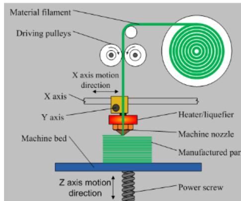
Figure 3. FDM process and its main components (Adel & Khalil, 2018).
