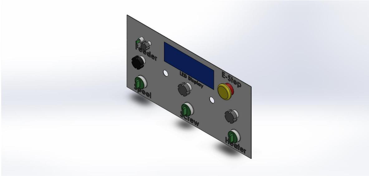
Figure 37. 3D CAD model representation of a Filament Extruder control panel (Own Work)
