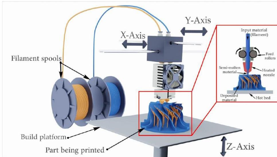
Figure 9. A diagram illustrating the FDM procedure (Elkaseer et al., 2020).
