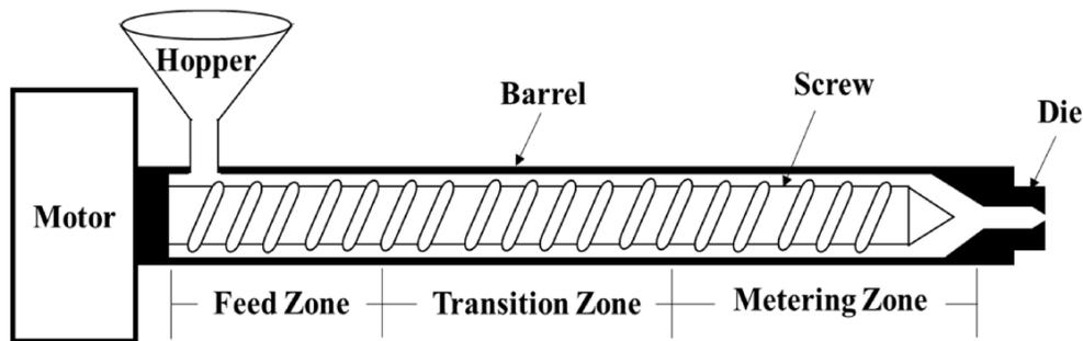
Figure 12. Shows a schematic layout representing barrel extrusion zones (Dey et al., 2021).
