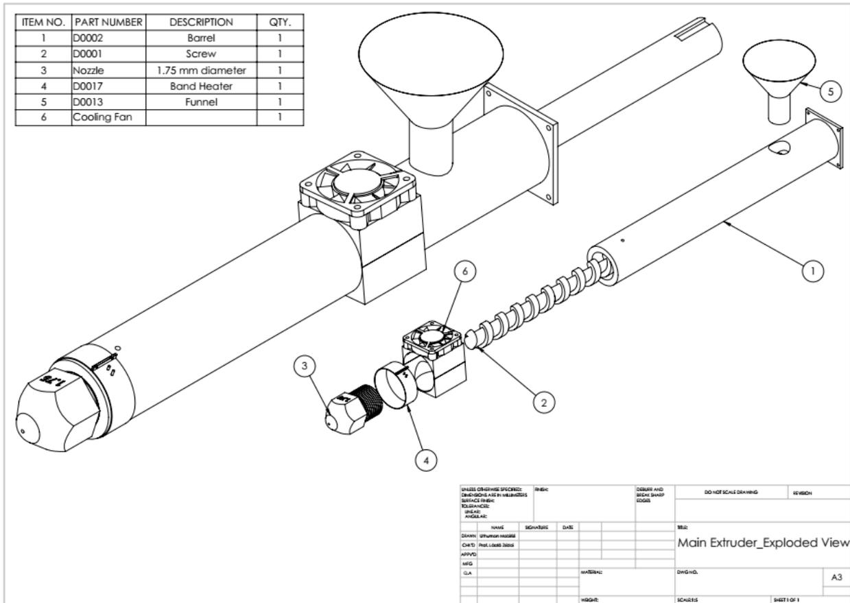
Figure 41. Exploded View of the Extrusion Section Assembly (Own Work)
