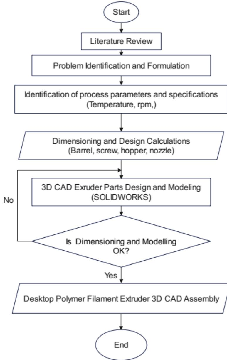
Figure 28. 3D CAD model Design Flow chart (Own Work)
