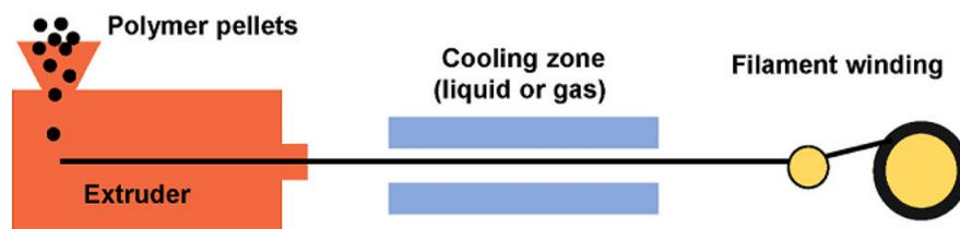
Figure 11. Feedstock filament fabrication process (Park & Fu, 2021).
