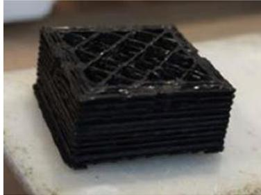
Figure 16. Losses in model layers (Sastri, 2022).
