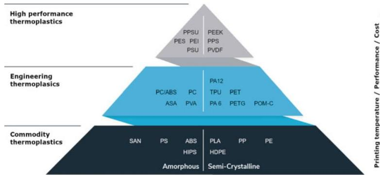
Figure 20. Thermoplastic material pyramid for FDM filament materials (Dave & Davim, 2021).
