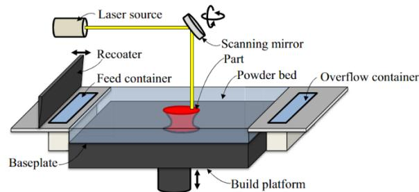
Figure 5. Selective Laser Melting process scheme (Yang et al., 2018).
