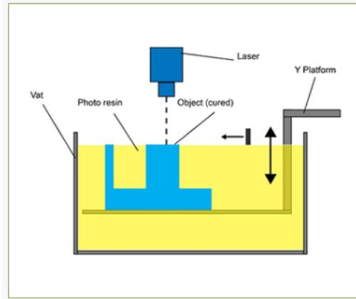
Figure 6. Stereolithography process scheme (Mathur, 2016).
