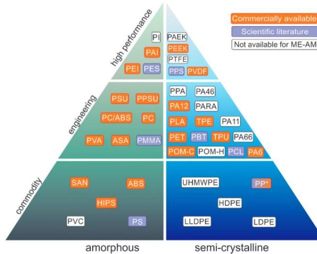
Figure 22. Polymeric material pyramid (He et al., 2014; Spoerk et al., 2020).
