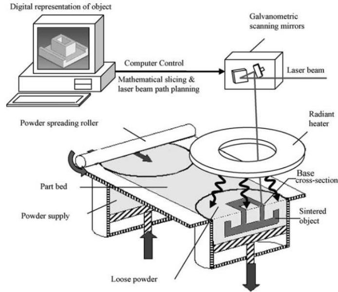
Figure 7. Selective laser sintering process scheme (Das, 2008).
