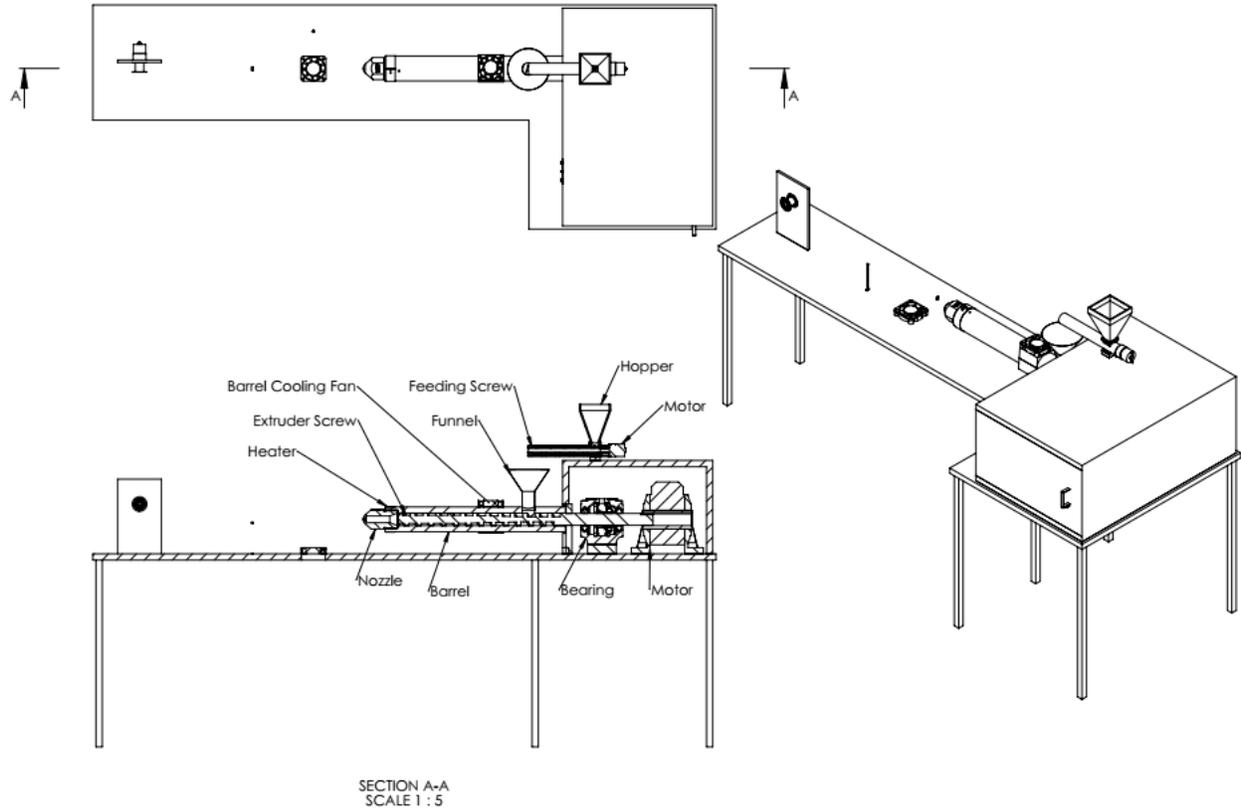
Figure 42. 3D CAD Model Design Assembly drawing view of the Desktop Filament Extruder (Own Work)
