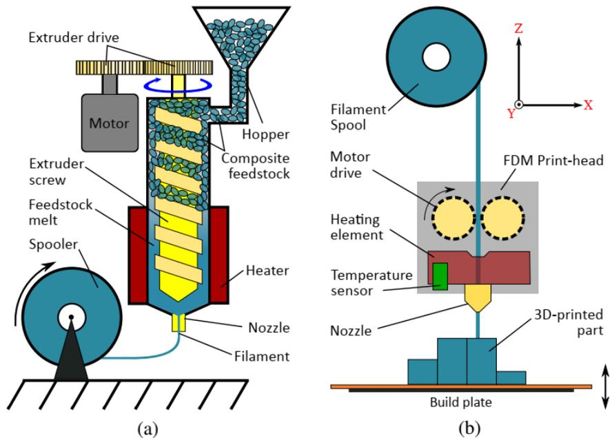
Figure 13. FDM filament fabrication and printing processes (Khatri et al., 2018).
