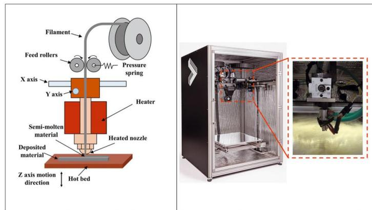
Figure 10. The FDM system's schematic view and actual representation (Zhang et al., 2019).
