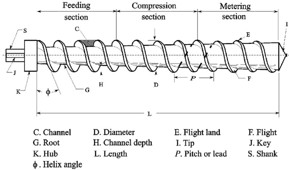
Figure 38. Geometric description of a single screw (Chan I. Chung, 2020).
