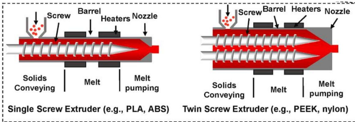
Figure 14. Schematic representation of Single and Twin-screw extruders (Park & Fu, 2021).
