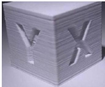
Figure 17. Visible waving of external surfaces of the model (Sastri, 2022).
