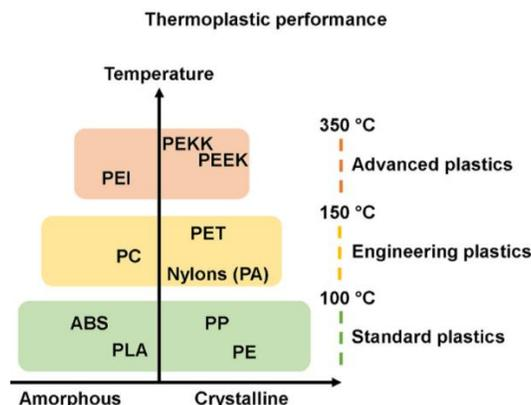
Figure 21. Typical thermoplastics are classified based on their performance (Park & Fu, 2021).
