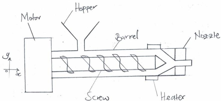
Figure 29. Horizontal layout of a filament extruder (Own Work)
