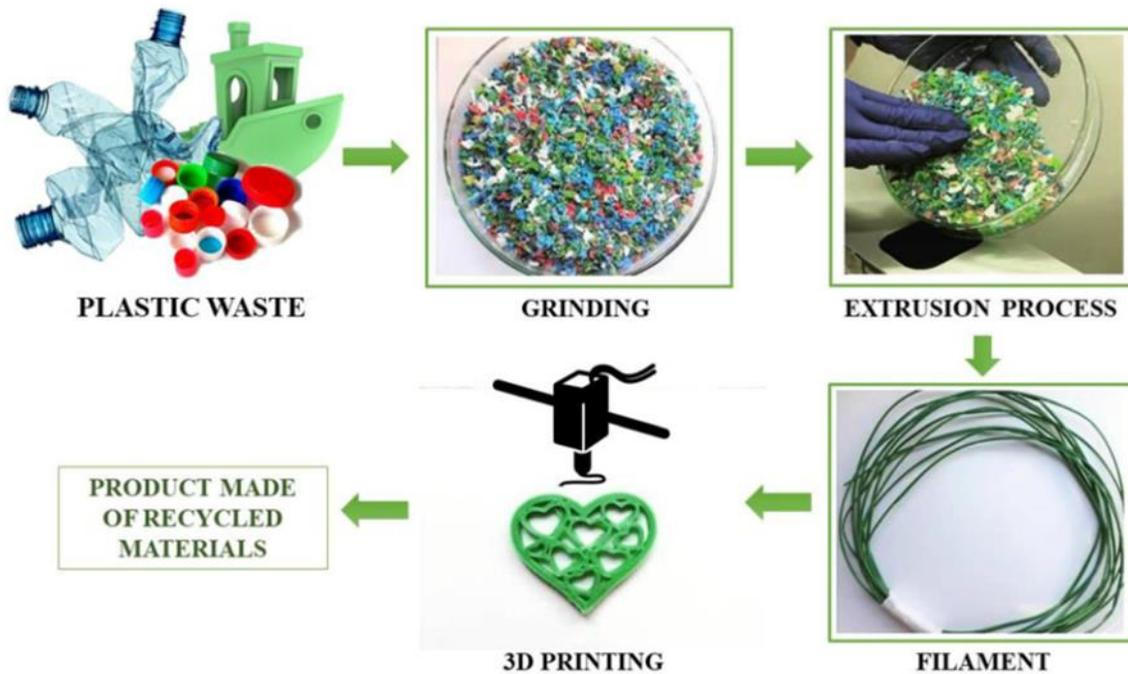
Figure 24. Material recycling system for filament fabrication (Mikula et al., 2020).
