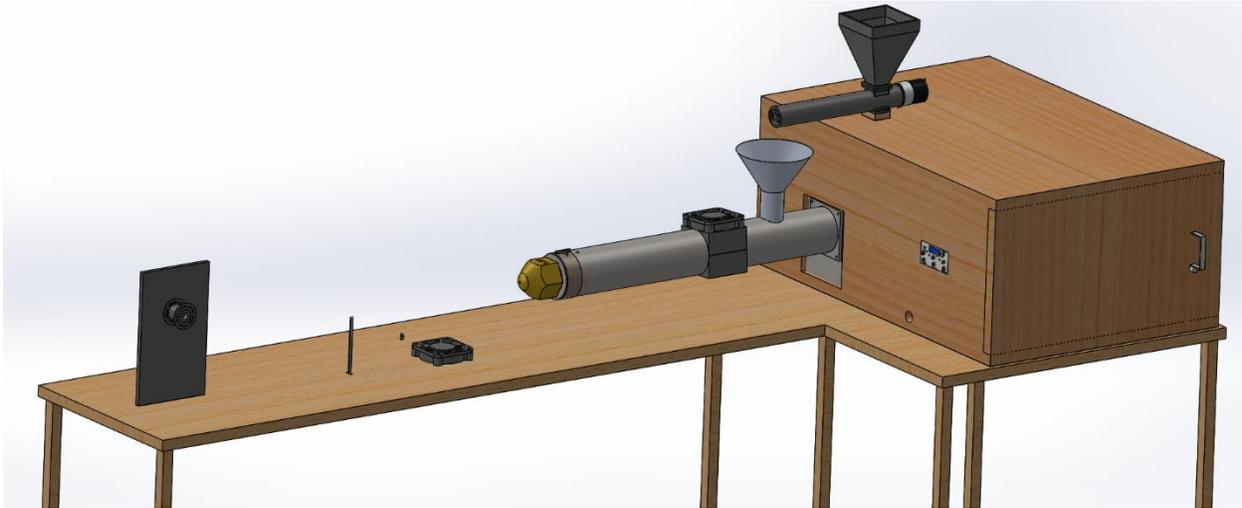
Figure 40. 3D CAD Model Design Assembly of the Desktop Filament Extruder (Own Work)
