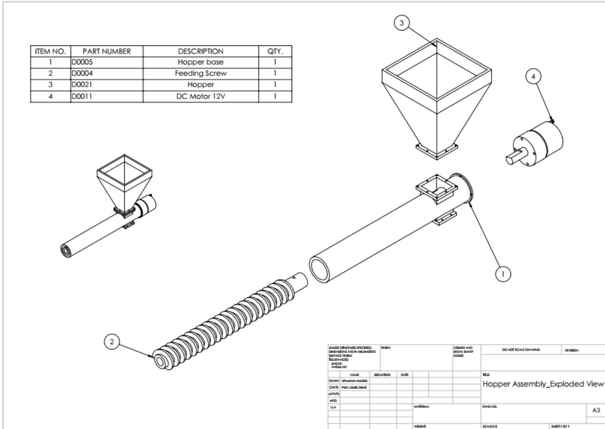
Figure 35. Hopper full Assembly exploded view (Own Work)
