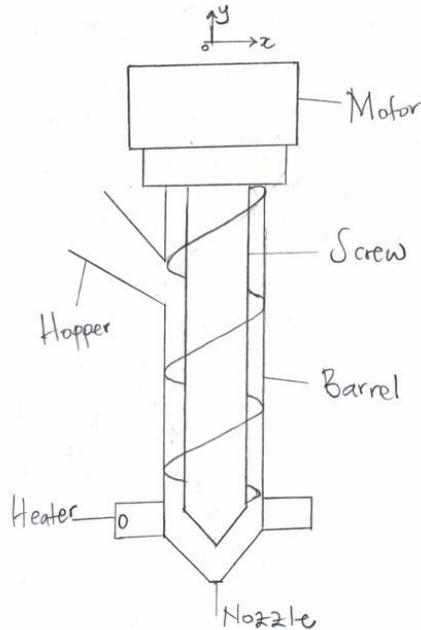
Figure 30. Vertical layout of a filament extruder (Own Work)
