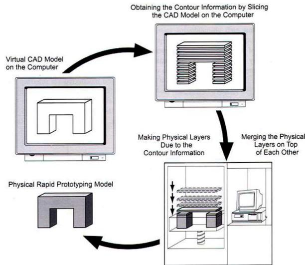
Figure 2. Rapid prototyping principle (Prakash et al., 2018).
