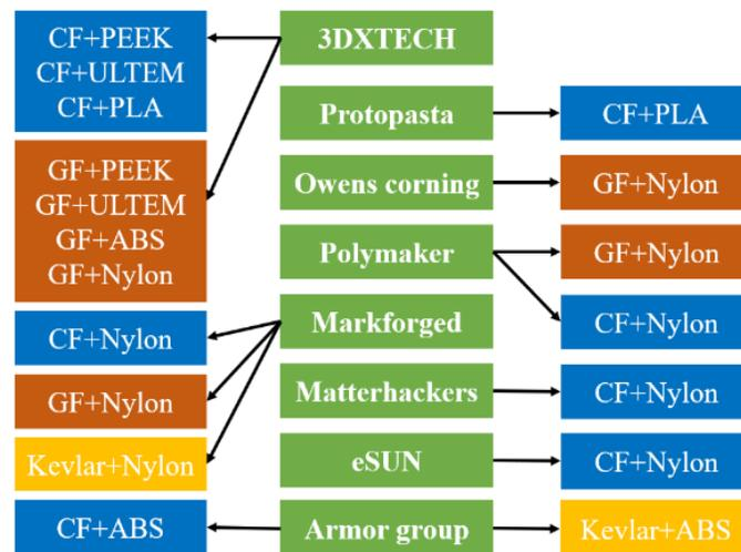
Figure 25. FDM fibre-reinforced composite filaments (Wickramasinghe et al., 2020).
