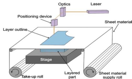
Figure 4. Laminated Object Manufacturing process scheme (Ahmad et al., 2019)
