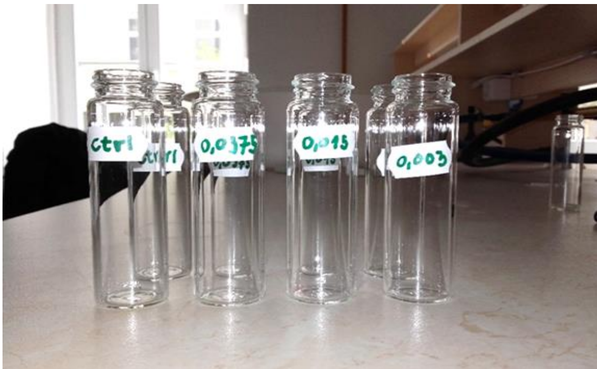
Figure 10 Glass vials with 2.27 cm diameter, 8.6cm length, 20ml glass vial (inner surface; 58.218 cm 2 )
