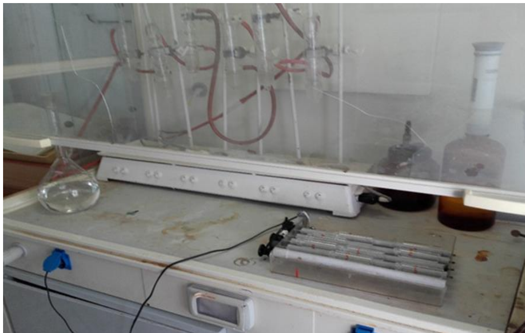
Figure 11 Rotation of the vials in a fume hood to vaporise acetone.
