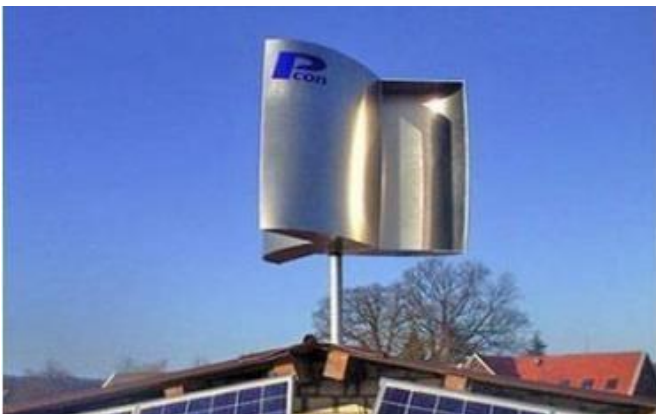
Figure 8: Savonius wind turbine (Wikipedia)
