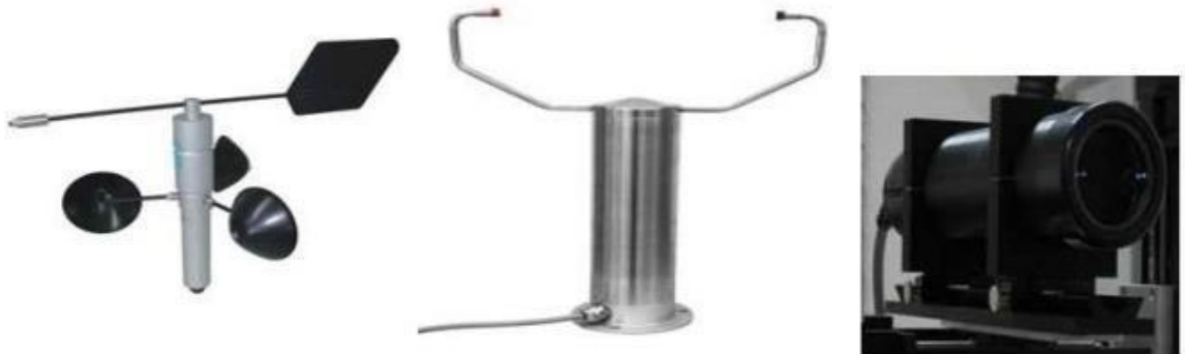
Figure 14: Anemometer: cup, ultrasonic and laser (Wikipedia)
