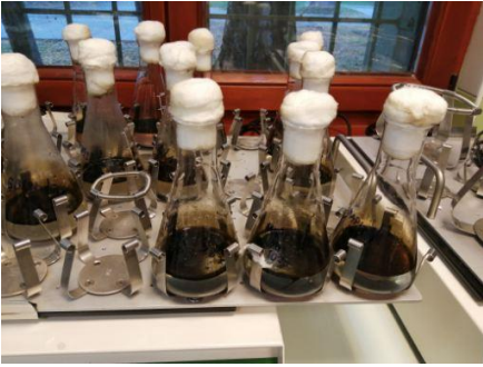
Figure 11. Incubated flasks on a shaker (120 h at 28 °C, 150 rpm) (Source: own work)
