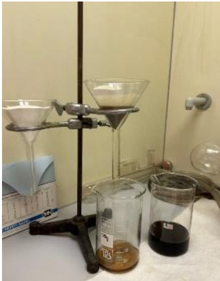
Figure 16. Phase filtration through filter paper to remove any residual water (Source: own work)
