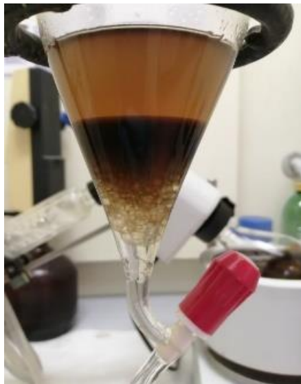
Figure 15. Formation of two phases: an aqueous phase and a petroleum-ether/oil phase (Source: own work)
