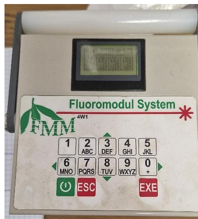
Figure 6. FluoroMeter Module (FMM) instrument used for chlorophyll-a fluorescence measurements in the algal growth inhibition test (Source: own picture)
