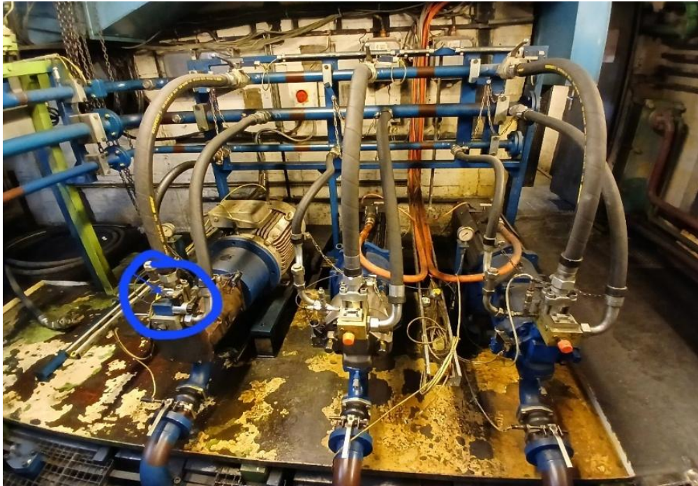
4. Figure: Sensor used for Hydraulic system of Ungerer line 3 (Source: Own photo , Arconic Székesfehérvár plant (2025))
