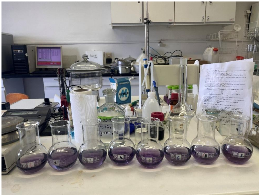
Figure 10: Color after titration with 0.05M H 2 SO 4
