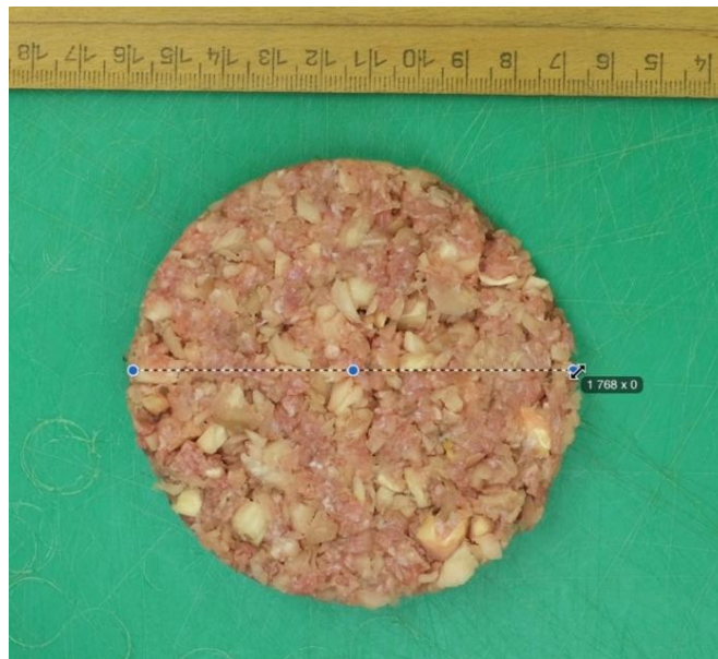
Figure 2.2 Representative picture of the visual shrinkage measurement process
