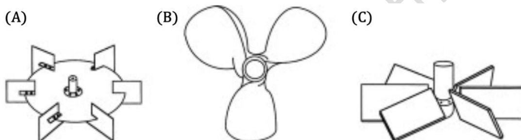
Figure 3. Schematic diagram of different types of impellers; (A) rushton turbine, (B) marine propeller and (C) pitched-blade turbine.
