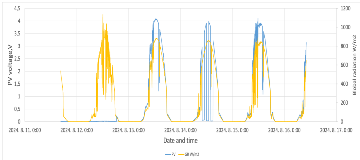
Figure 15 Effect of shadow on PV output and global radiation
