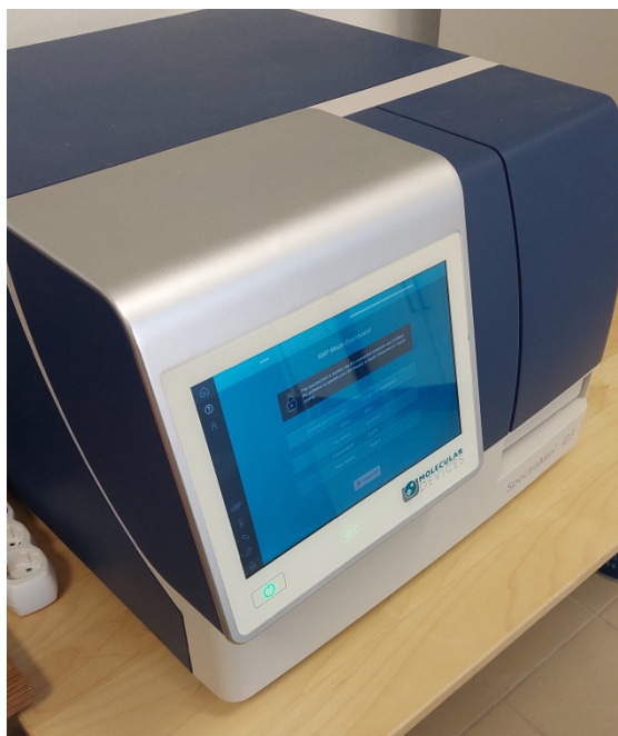
Figure 8. SpectraMax iD3 Multi-Mode Microplate Reader (source: own photo)
