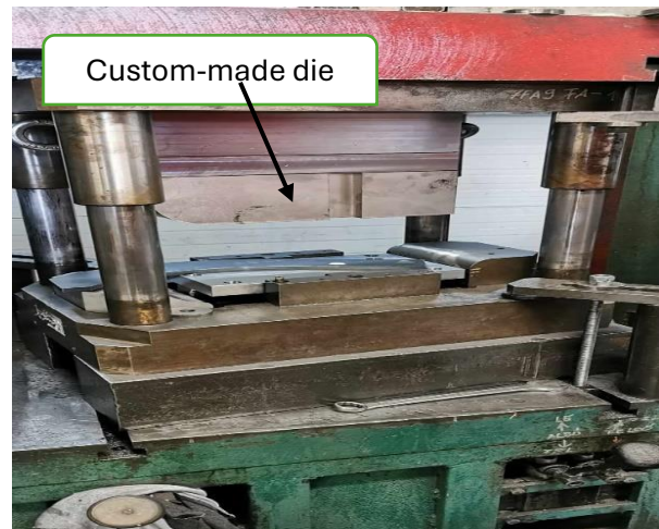
Figure 14; Press or Shaping Machine (our own pic.)
