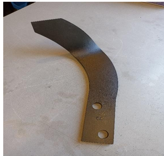
Figure 15: Blade After shaping (own pic.)
