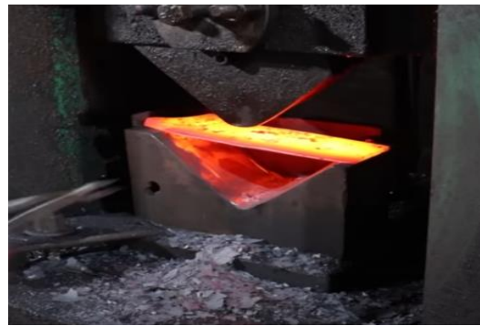
Figure 17: Shaping in a press.
