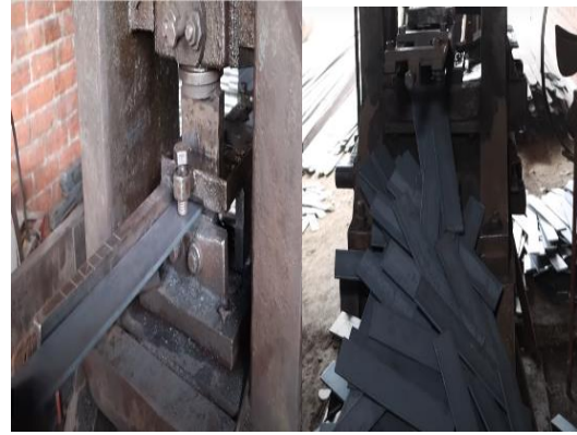
Figure 11: Cutting in required pieces. (own pic)
