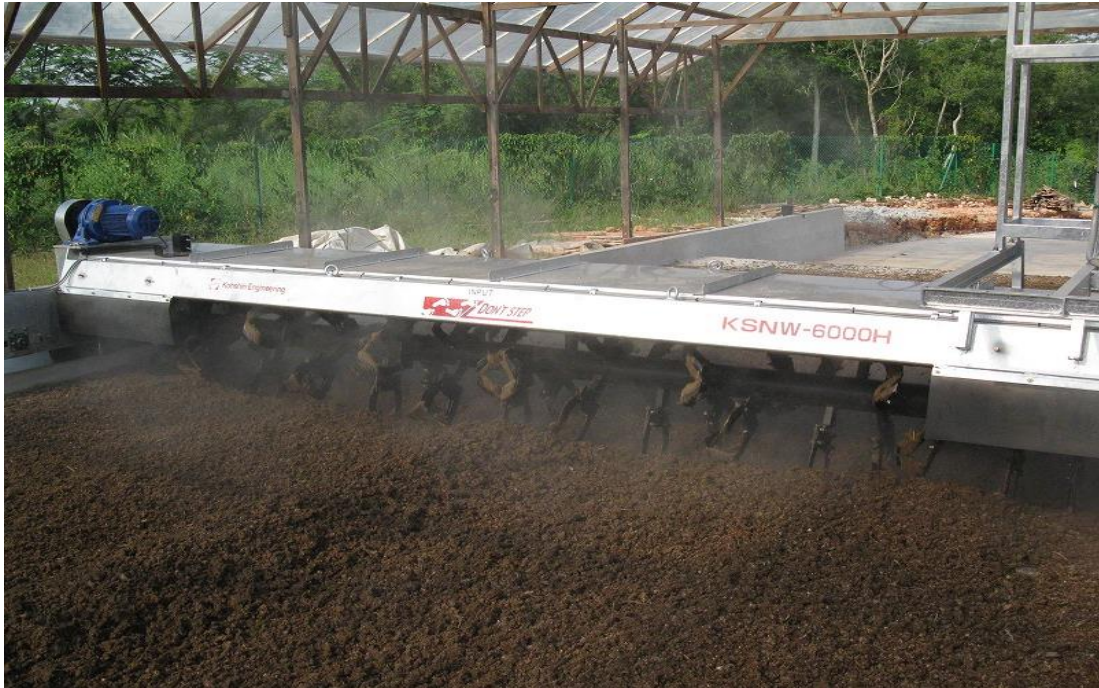
Figure 7: KSN machines (Dryer and semi-composter) https://www.kohshin-s.jp/product-en/ksn-type-fermentation-dryer/
