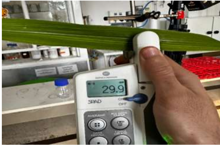
Figure 11: Measuring pigment content by using SPAD
