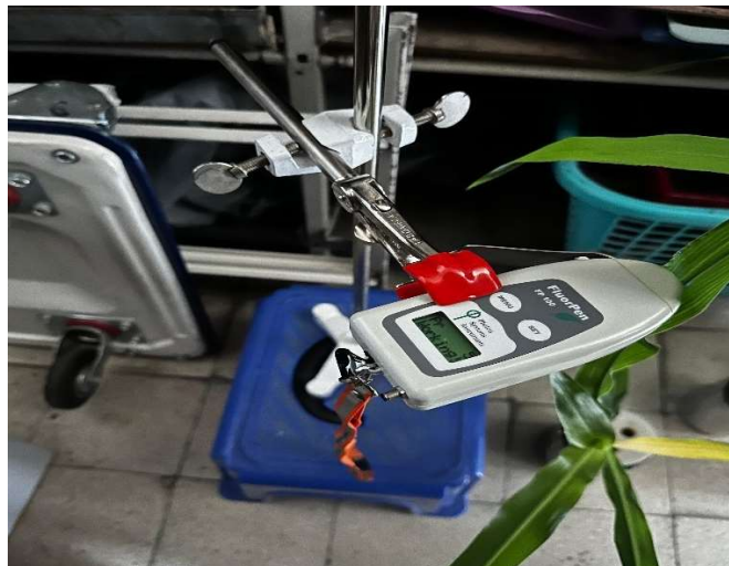
Figure 12: Measuring chlorophyll fluorescence by using Fluorpen
