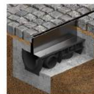
Gutter line details
