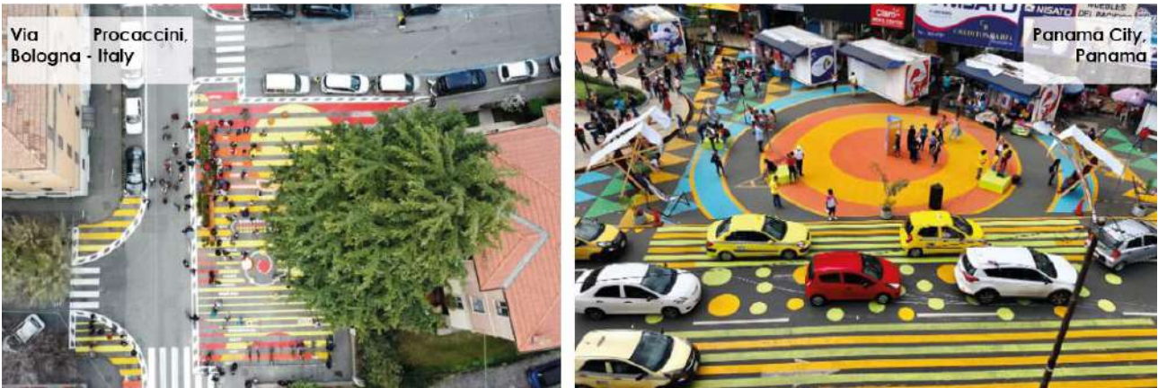
Figure 22. Examples of existing Tactical urbanism solutions in slip lane closure
