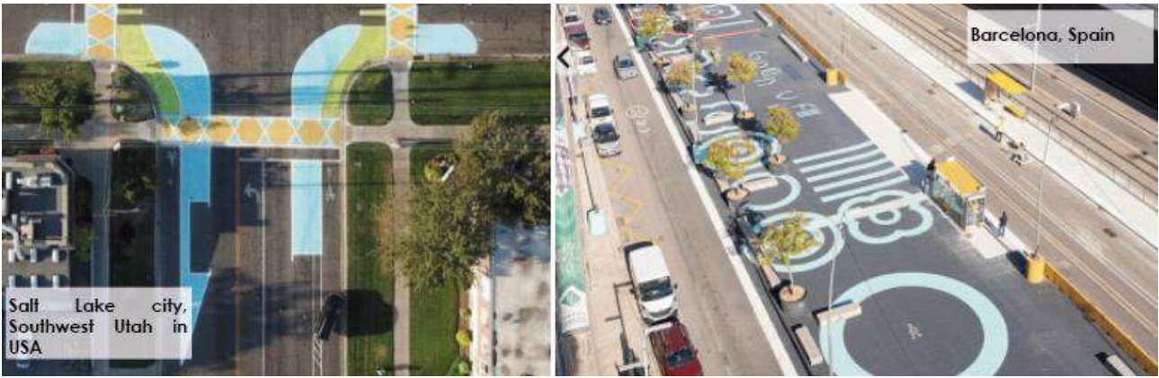
Figure 21. Examples of existing Tactical urbanism solutions in Lane narrowing
