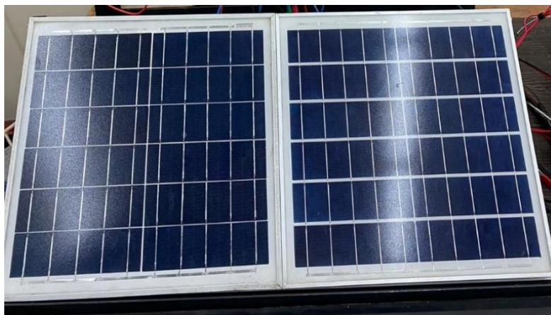
Figure 4-32: 6-volt 2.5-amp solar panel
